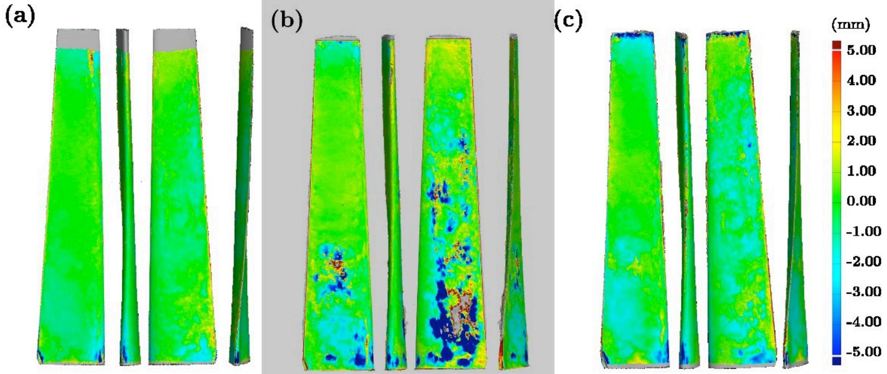
Deviation maps of the reconstructed model captured in different light intensity
